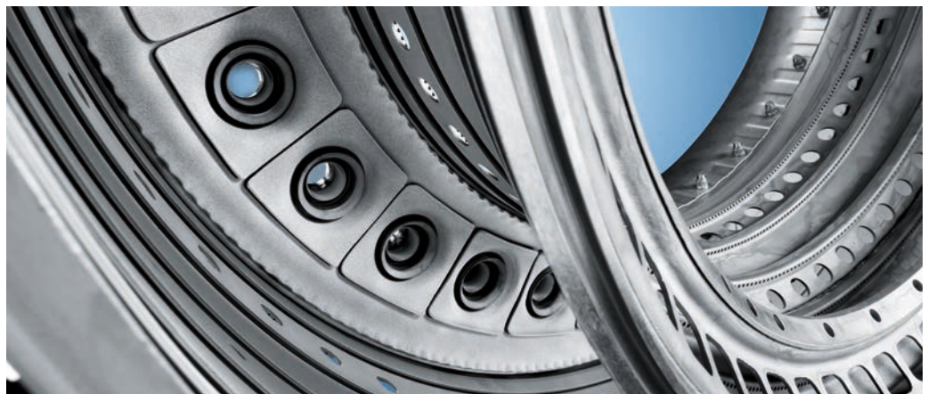
A combustor after being fitted with a new insulation layer: with in-depth repairs, MTU Maintenance aims to ensure that components enjoy a long service life
