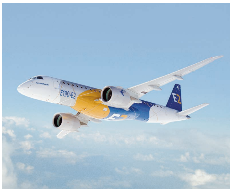
Certified in 2017: the PW1900G for the new generation of E-Jets from Embraer. Thanks to the Geared Turbofan™, the E190-E2 consumes 17 percent less fuel and thus produces 17 percent less CO 2 .
